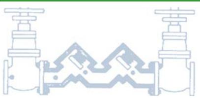
**CROSS-CONNECTIONS.** The City has a comprehensive Cross-Connection Control Program. Backflow prevention assemblies are inspected, tested, maintained, and/or repaired annually to ensure required protection is provided. Potential cross-connections are identified and eliminated or protected by a backflow preventer.
